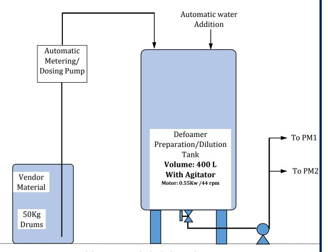
Separate delivery pumps for both the Machines.
