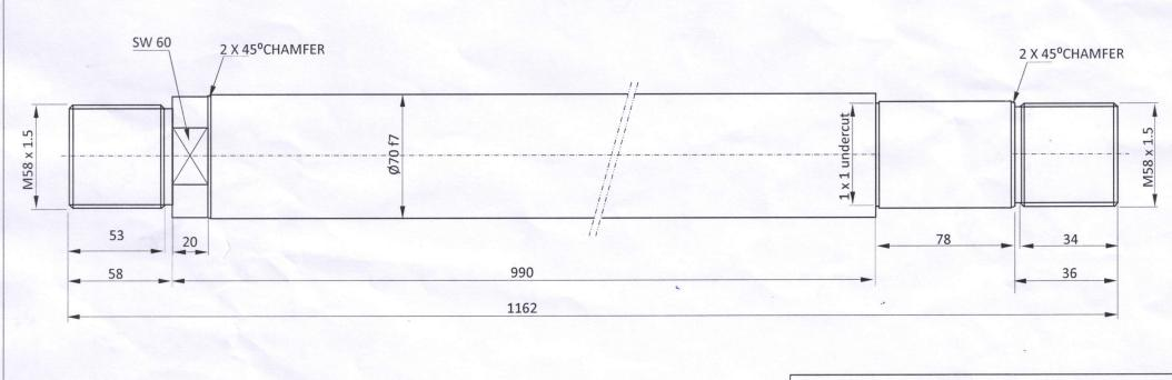
ALL DIMENSIONS ARE IN MM UNLESS UNTIL SPECIFIED HARD CHROME COATING OF 30µm to 50µm REQUIRED
