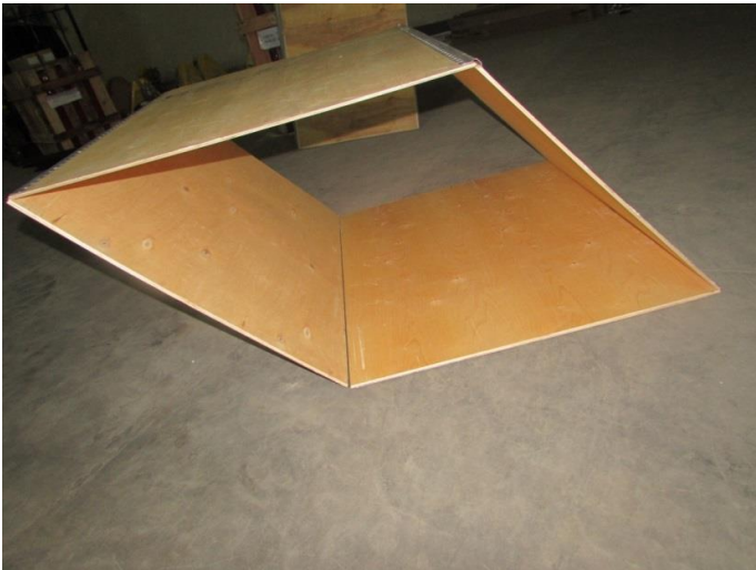
COLLAPSED CONDITION OF SIDE COVER (indicative fig)
