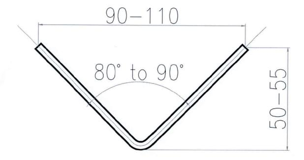
REINFORCEMENT ROD 4 mm DIA.
